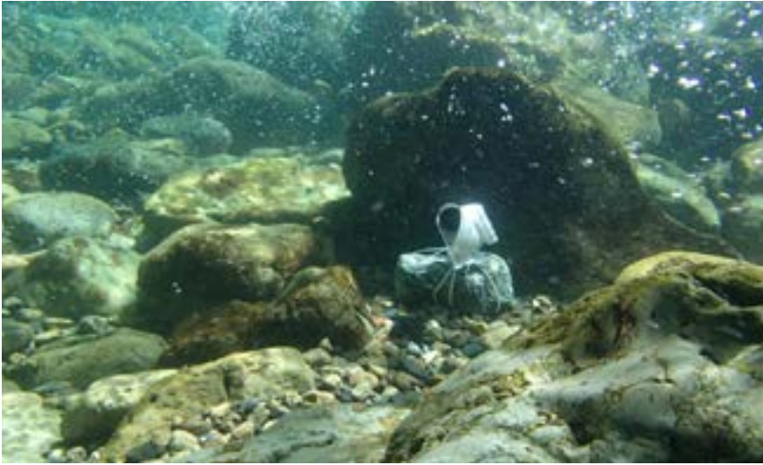
A temperature logger deployed in a stream. Loggers are attached to weights or rocks to suspend them within the channel.
