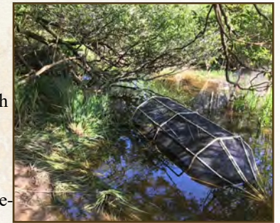
A hoop trap set in Kermit Creek to monitor juvenile coho use.
